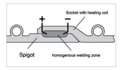
Fig. 4 - Welded joint - schematic representation; integrated E-socket
