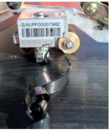
Fig. 8 - Peeling of the pipe surface before electrofusion DN/ID 1200 mm
