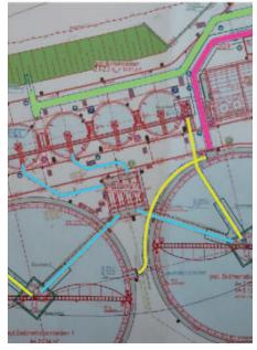
Fig.1 - Overview of the construction project, contact and sedimentation basin with connecting pipes made of PE 100
