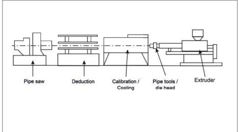
Fig. 5 - Production of PE pipes according to DIN 8074/75 - Pipe extrusion line schematic
