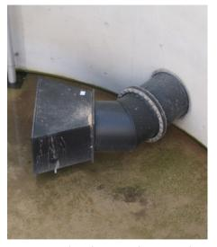
Fig. 11 - Flanged transitions from rectangular to round DN/ID 900 mm made of PE sheets
