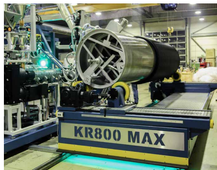
Picture 8: A test pipe on the new machine
