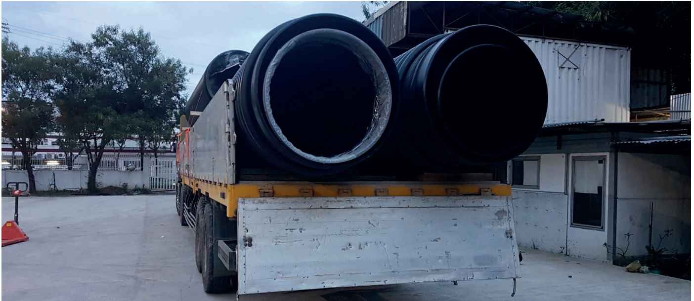
Photo 1: Loading of 800mm diameter pipes inside 1000mm diameter pipes, first delivery to Nuvista San Jose project site
