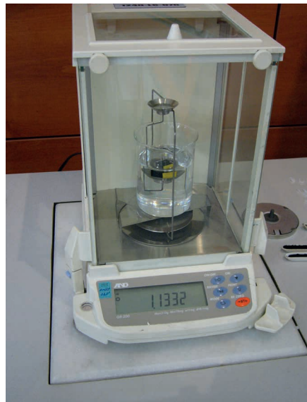
Photo 8: Device for density determination
