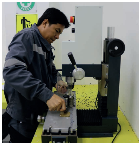
Photo 3: Preparing the test specimen from a pipe
