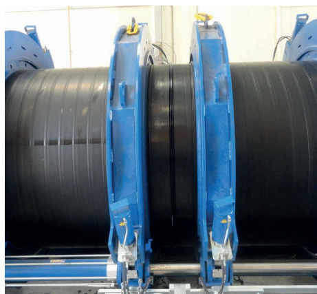
Photo 1: Krah pressure pipe, spiral wound acc. to DIN 16961. Source: UGPM, Sultanate Oman
