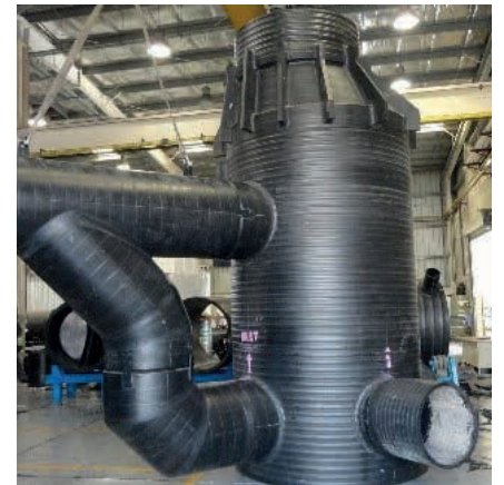
Photo 9: Prefabricated Krah manhole
