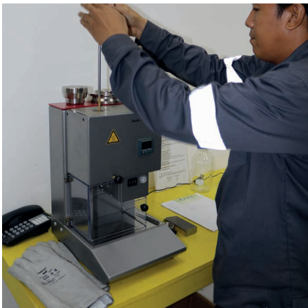
Photo 7: Device for testing of the melt flow rate (5)
