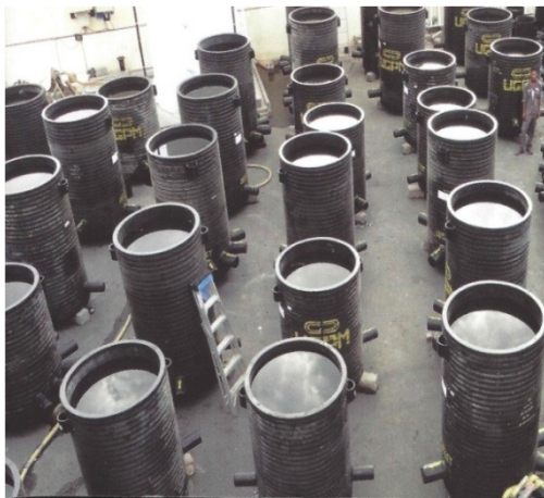
Figure 7: Krah HDPE Manholes at Hydrostatic test
