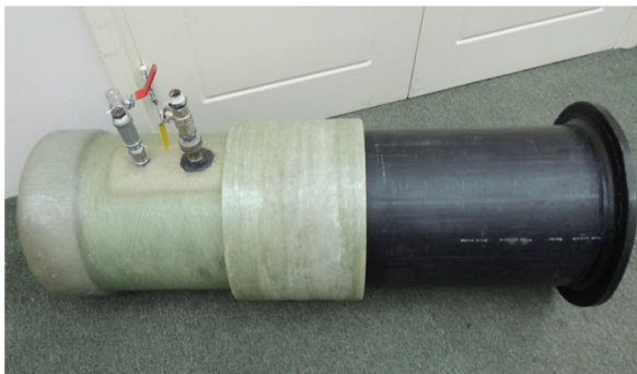
Figure 12: HDPE to GRP, including test unit
