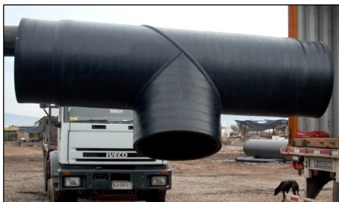
Pic1: Butt-fused T-piece with increased wall thickness
