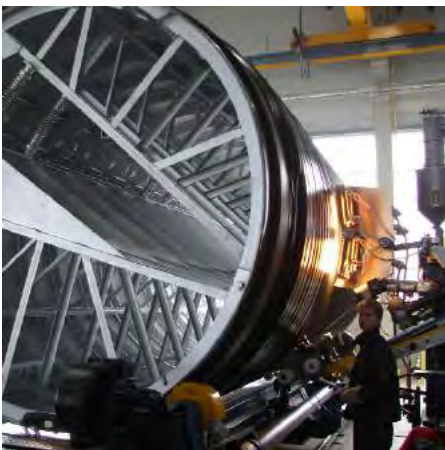
Production line KR800-MAX able to produce KMP up to DN/ID 4000 mm
