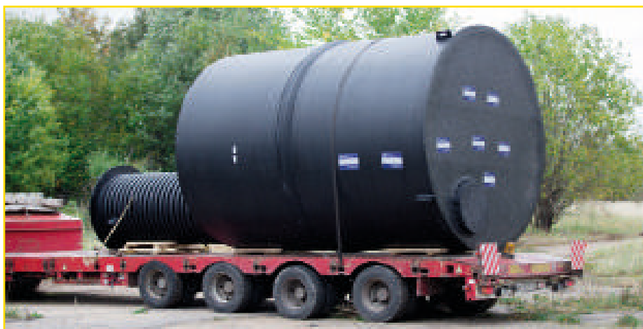
Fig. 1. The appearance of the water tower tank
