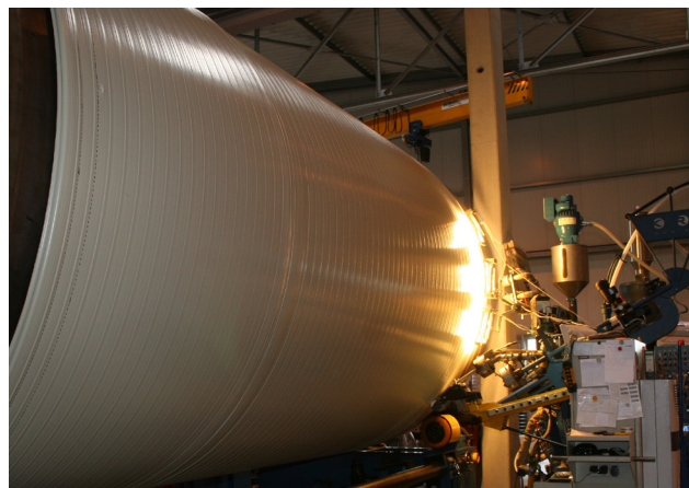
Polypropylen tank production DN 2700 with stepped wall thickness
