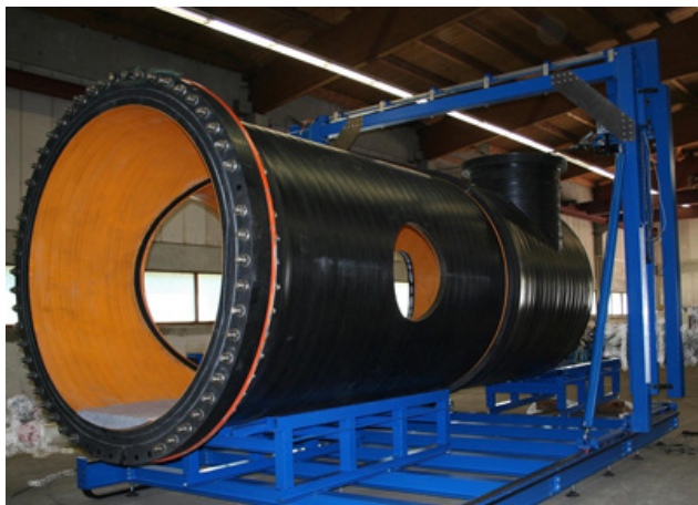
Joining the 1050 mm diameter pipes by electro-fusion
