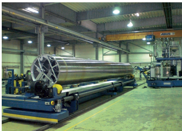
Krah has developed a special procedure for extending the old 7 m long mandrels to 13 meters.
