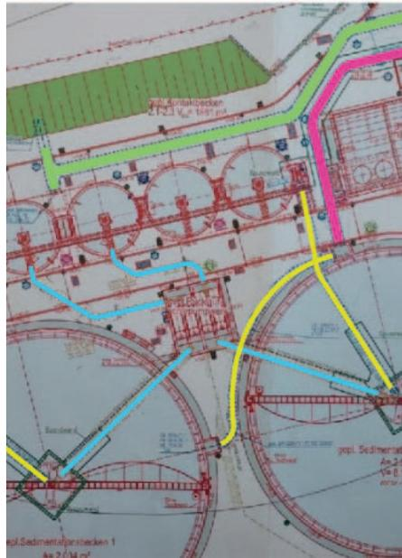
Fig.1 - Overview of the construction project, contact and sedimentation basin with connecting pipes made of PE 100
