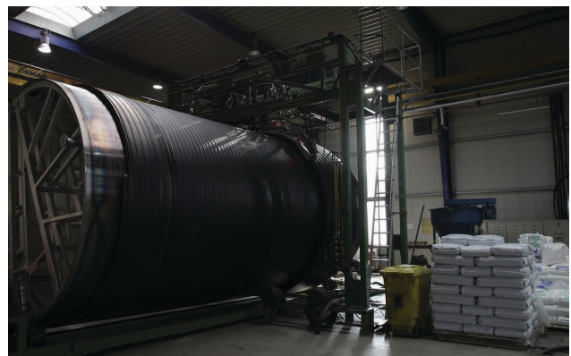
Pipe production / helical extrusion process
