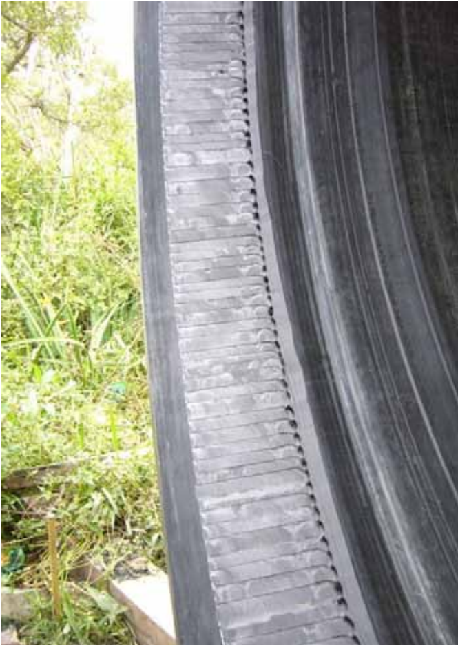
Finished surface of socket
