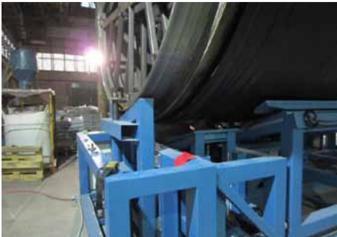
Reinforced machine and mandrel in production hall
