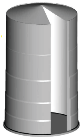
Tiered cylindrical tank made of a helically extruded pipe
