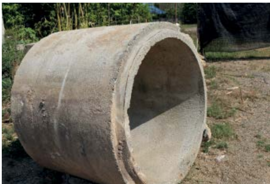
Pic. 3: Concrete pipes with high roughness and socket (Source: Krah Pipes GmbH & Co. KG)
