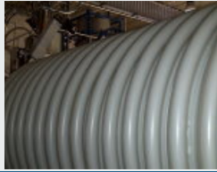
Advantages of using High Modulus Polypropylen for gravity pipes
