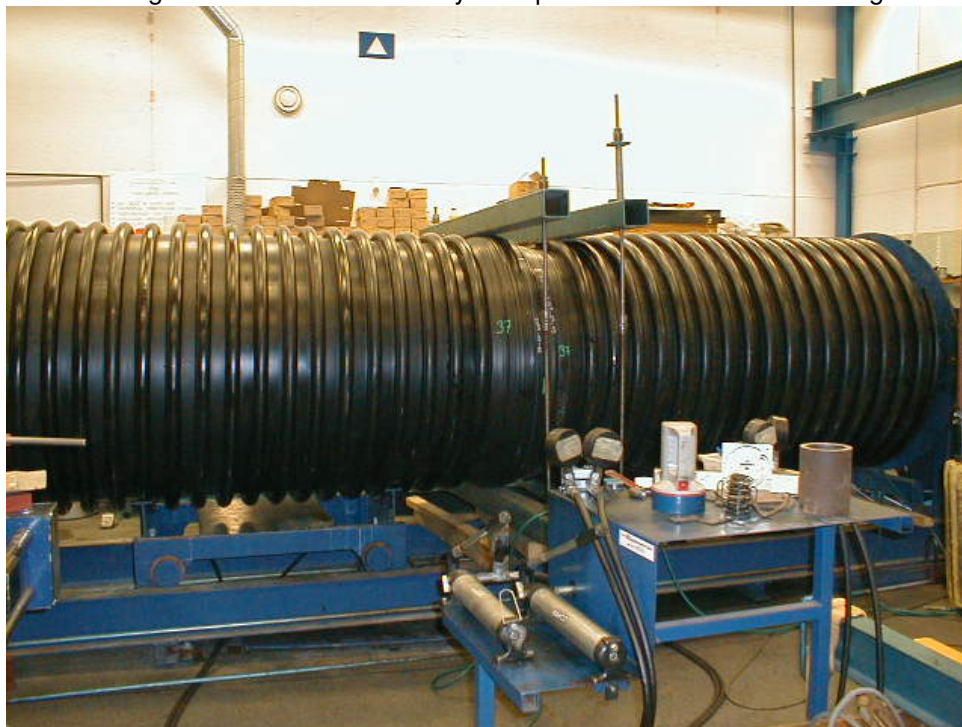
Dn1200mm pipe joint during EN1277 condition B testing at our test laboratory.
