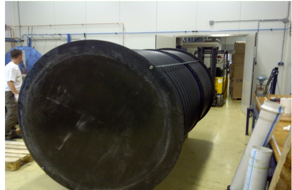
Dn1800mm Pipes with welded end plates
