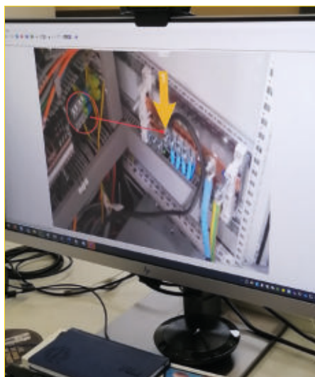
Pic. 11: Our operator can draw in the screen. The one wearing the AR-glasses sees this.
