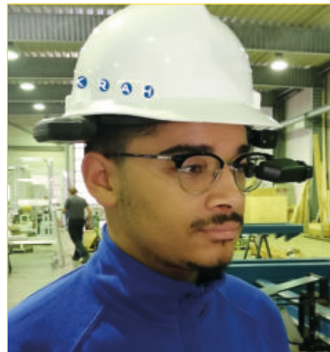
Pic. 7: The AR-glasses are integrated in a safety helmet.
