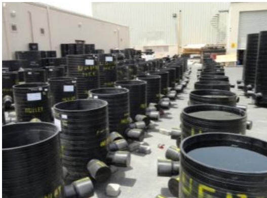
Pic 6: Test of water tightness acc. DIN EN ISO 13598; 100% Control at UGPM,Oman
