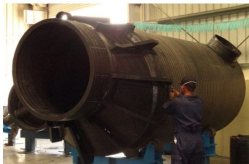
Pic 5: Fabrication of PE100-Sewer Manhole at UGPM (DN1600/1200, with cone, height 3800 mm)
