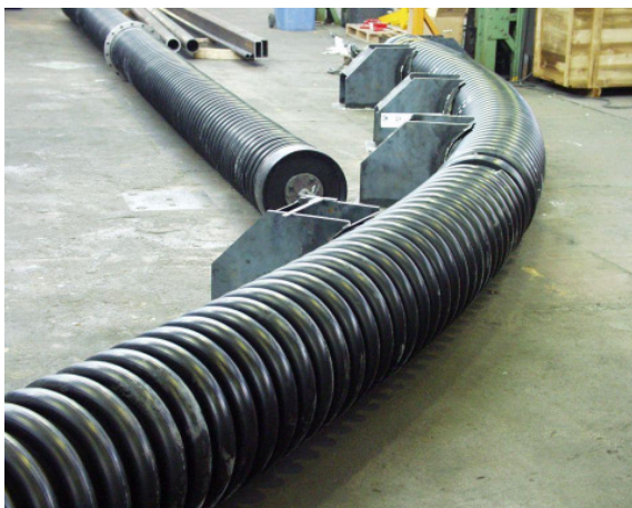
Bending test, profile-pipe
