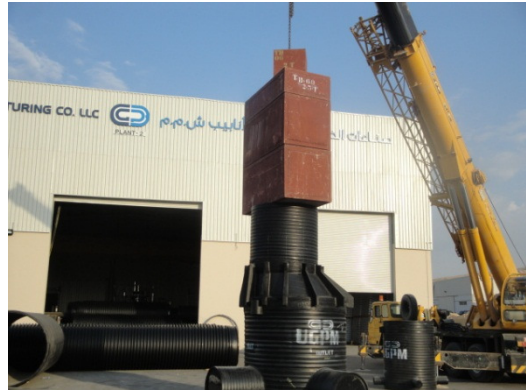
Pic 7: Test of vertical load acc. DIN EN ISO 14802 (special test set-up for large diameter manholes, not buried in soil-box, UGPM,Oman)
