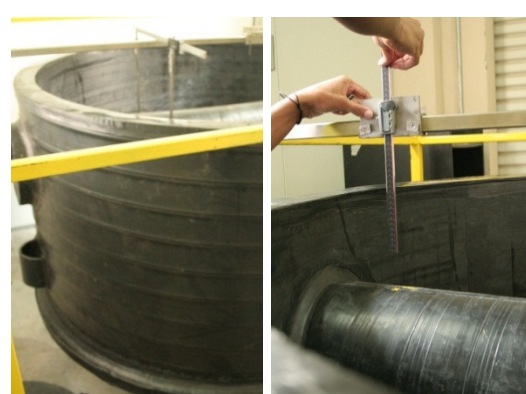
Pic 9: Test of structural integrity acc. DIN EN ISO 14830, vacuum test at 20 °C, free assembled test set-up
