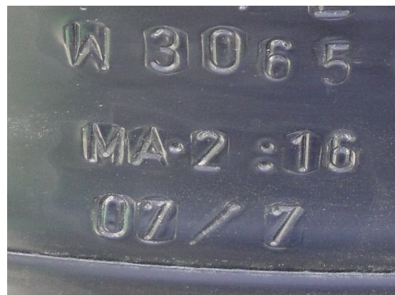
Pic 10: Traceability code at welding joints, stamped welding seam, UGPM, Oman)
