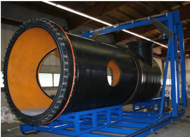
Joining the 1050 mm diameter pipes by electro-fusion
