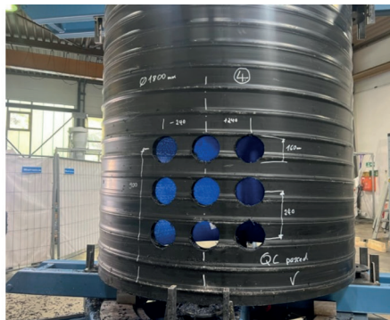
Figure 2: Multi object mode. Object definition on machine panel (left) and processed pipe (right).
