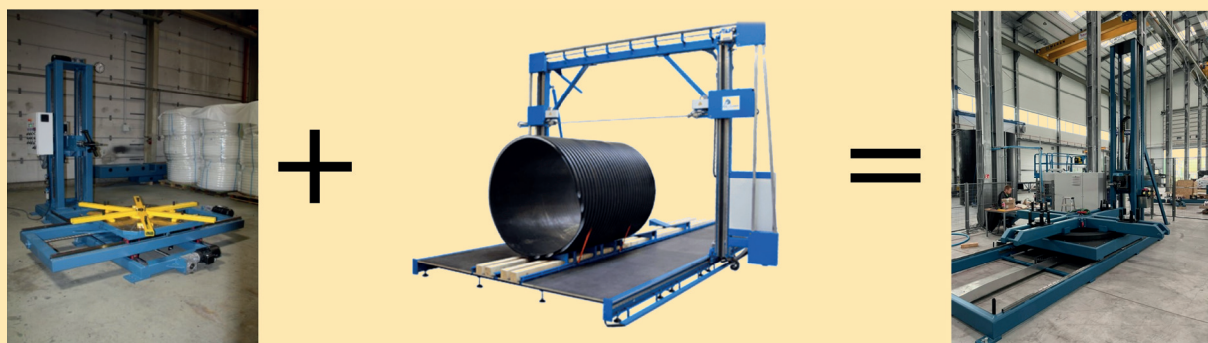
Figure 5: Comparison of functionality. Conventional milling station MF-200 (left), saw machine from Eugen Riexinger GmbH & Co. KG* (middle) and new MF-400 CNC milling station (right).
