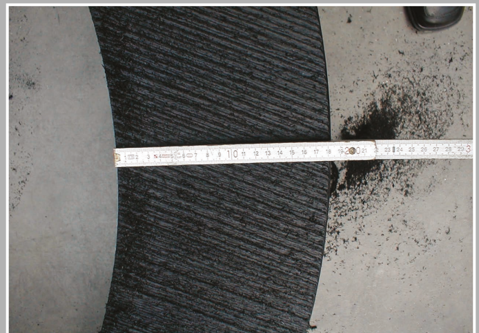
Solid wall polyethylen pipe, s = 180\text{mm} (7")
