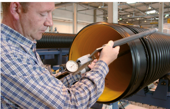
Checking of the wall thickness
